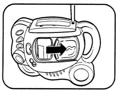
I. Slide lens cover open if necessary. Use a Phillips screwdriver to loosen screw securing compartment door and remove door (screw will remain attached to door).
